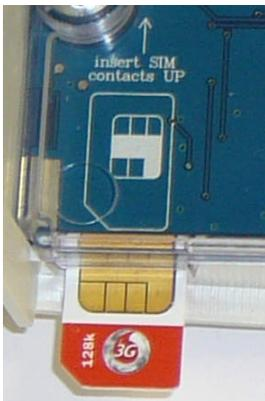
Insert SIM card with the contacts upward and chamfered corner at the lower left.
